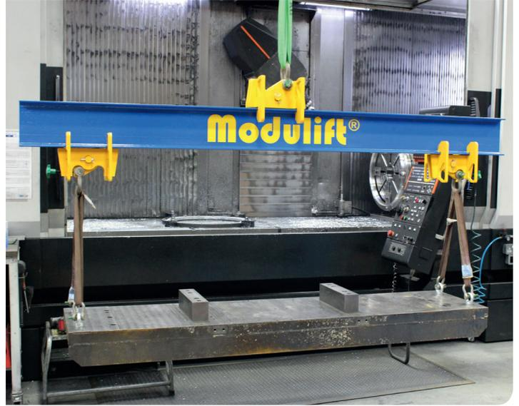
Fig. 2) Lifting beam configuration
